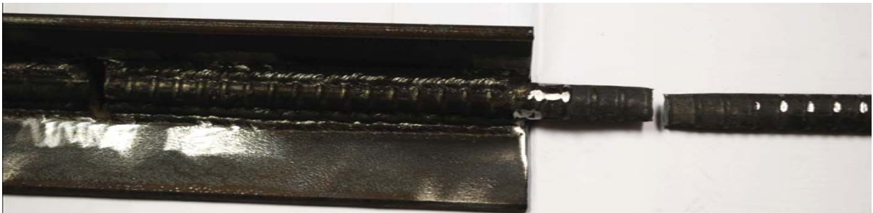
A tensile test was performed to verify that the integrity of the material was not compromised (a 500°F preheat and interpass temperature was maintained).
